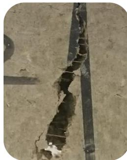
Crack pattern in SBF-reinforced earth block
