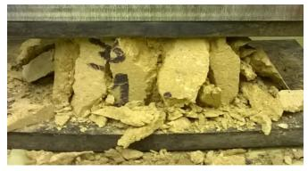
Specimen after compression test
