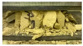
Specimen after compression test
