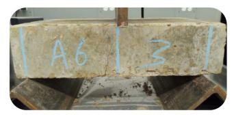
Flexure test of unreinforced earth block
