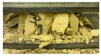
Specimen after compression test
